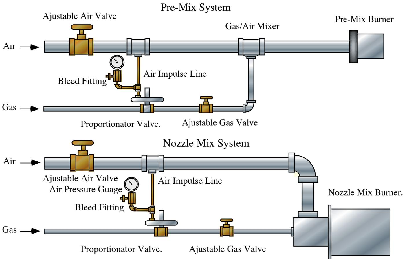
The system is now set up for manual single valve control of the furnace firing range. To turn the furnace up, open the main air valve. To turn it down, close the valve. Now we can install a programmable controller and motorized air valve to control the firing of the furnace.
